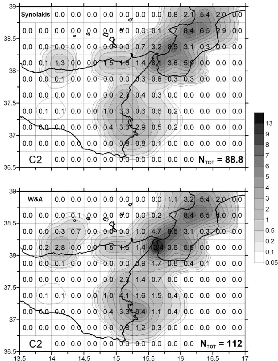
Fig. 7 Catalogue C2 contour plots, and cell-by-cell and cumulative number of tsunamigenic earthquakes expected to generate tsunami waves with coastal heights larger than 1 m along any coastal segment in 10,000 years ( $N_{TOT}$  is the total number of expected events in the entire region)
