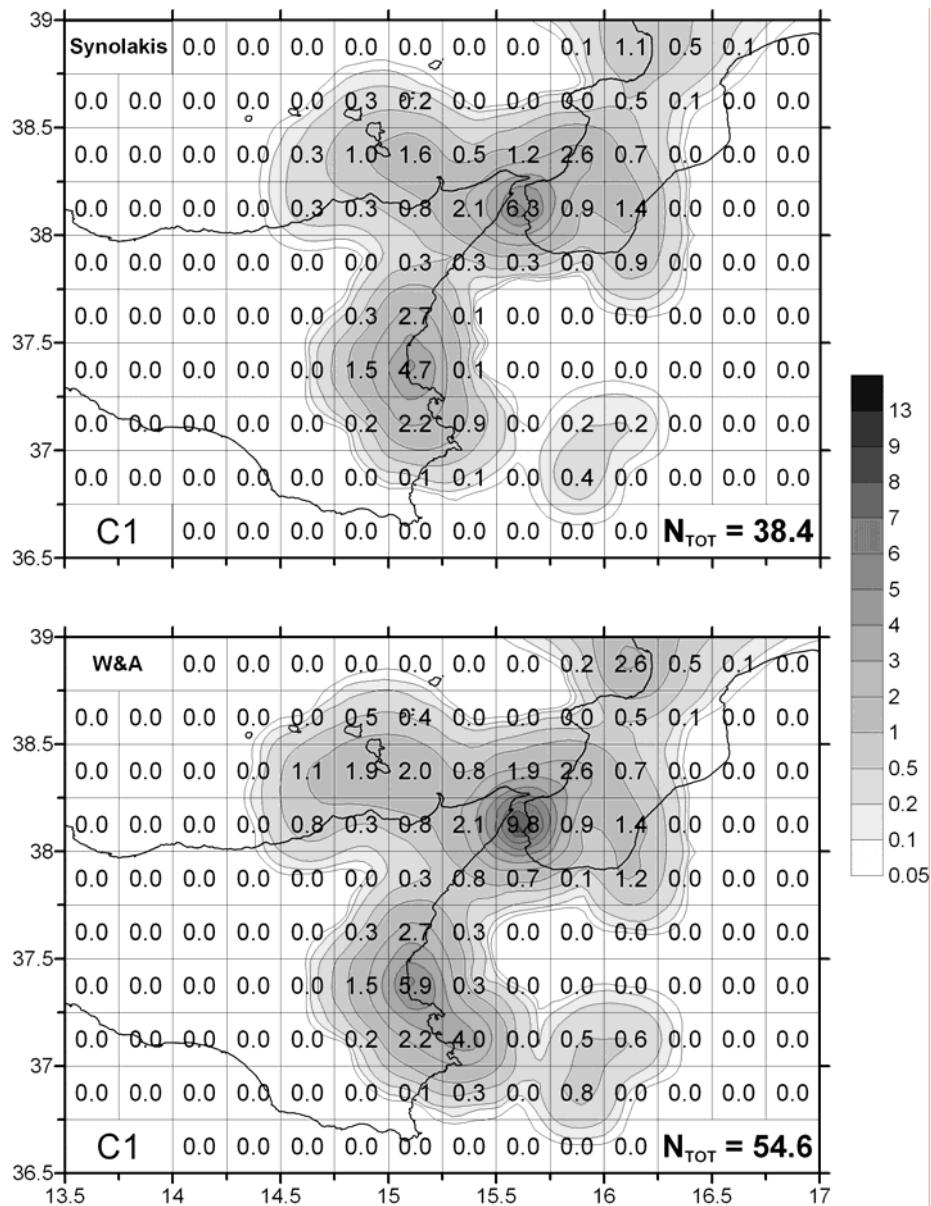
Fig. 6 Contour plots, and cell-by-cell and cumulative number of tsunamigenic earthquakes expected to generate tsunami waves with coastal heights larger than 1 m along any coastal segment in 10,000 years (the results refer to the catalogue C1;  $N_{TOT}$  is the total number of expected events in the entire region)
