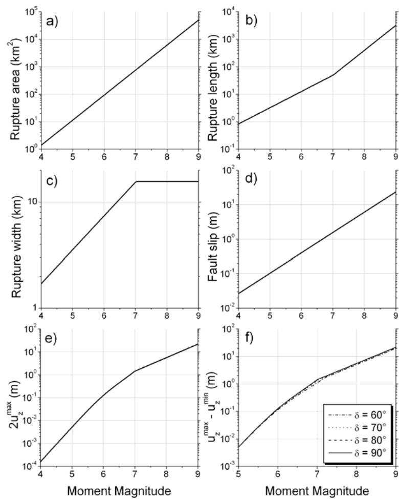
Fig. 5 (a) Area, (b) length, and (c) width of the faults as functions of the earthquake moment magnitude, computed through Wells and Coppersmith (1994) empirical relationships, (d) Uniform slip on the fault computed through Hanks and Kanamori (1979) formula and through the definition of scalar seismic moment, (e) Maximum vertical offset as a function of earthquake magnitude for vertical dip-slip faults, (f) Dependence of the maximum vertical offset on the dip angle of dip-slip faults
