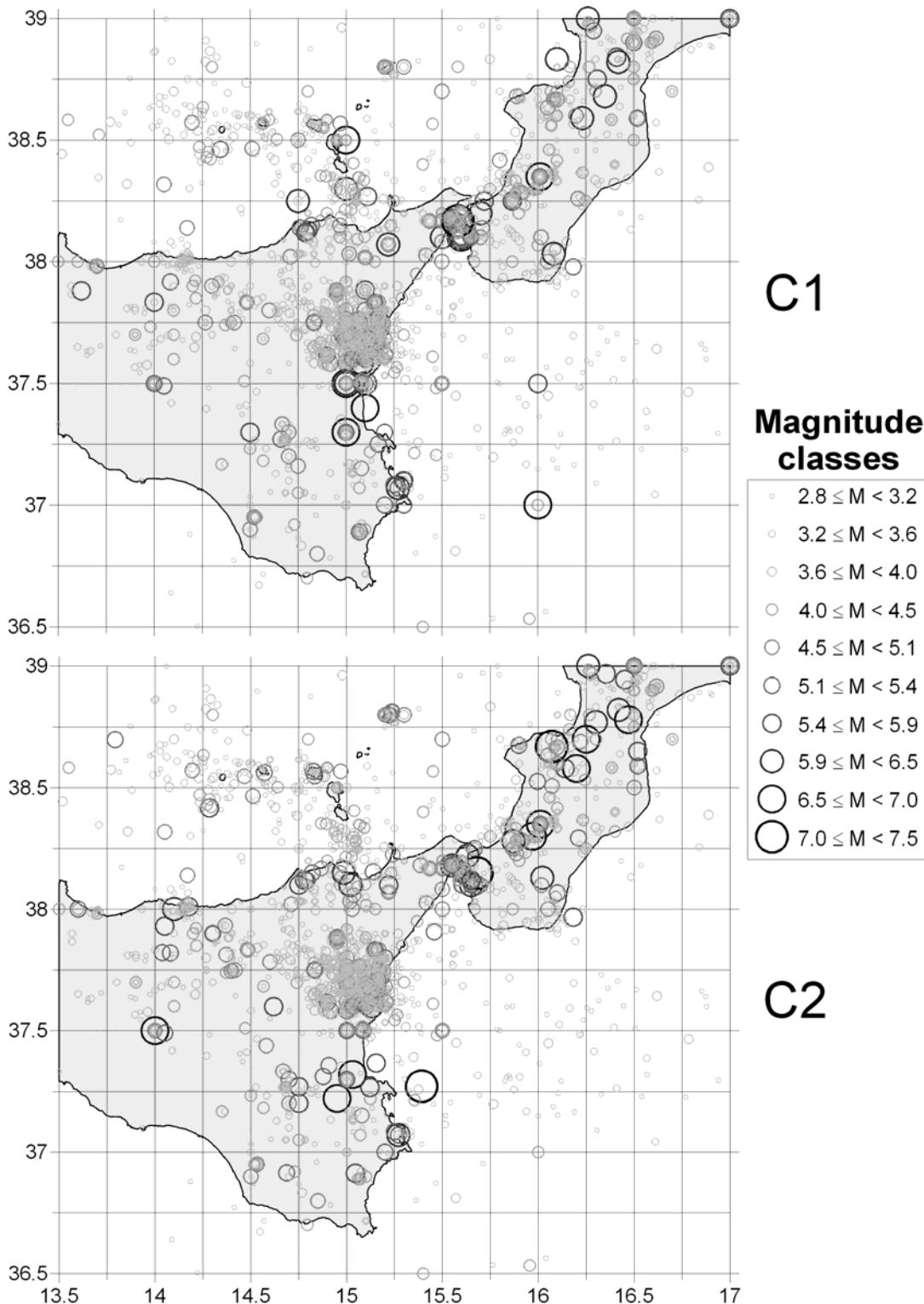
Fig. 2 Distribution of the earthquakes contained in the catalogues C1 and C2 (events belonging to different magnitude classes are plotted with different sizes; the magnitude classes are the same as used in the statistical analysis, with the exception that in the analysis the last two classes are combined together)
