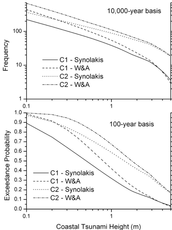
Fig. 8 Dependence of the number of events expected in 10,000 years (upper plot) and of the probability of exceedance in 100 years (lower plot) on the coastal tsunami height (the probability estimation is based on the assumption that the occurrence of the tsunamigenic earthquakes is a Poissonian process)
