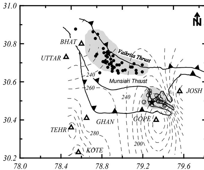
Fig. 8 Contours of  $Q$  prepared from the obtained values of  $Q$  at different stations on tectonic map of the region (shaded circles show the rupture areas of the two earthquakes; shaded regions show the aftershock areas; the aftershock data of the Uttarkashi Earthquake is taken from Kayal et al. (1995) and that of the Chamoli Earthquake from Mandal et al. (2001))
