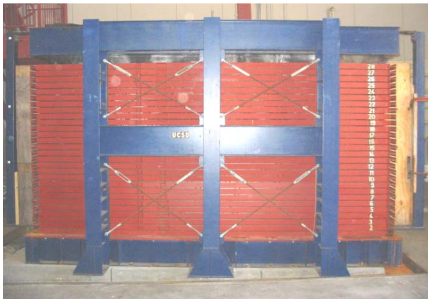
Fig. 4 The UCSD medium size laminar box (Jakrapiyanun, 2002)
