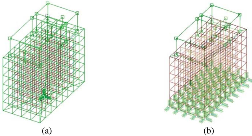
Fig. 5 Various methods of soil representation for FE modeling: (a) soil represented by a set of three translational springs,  $k_x$ ,  $k_y$ ,  $k_z$ , and three rotational springs,  $k_\theta$ ,  $k_\psi$ ,  $k_\phi$ , applied at the CG of the base of the foundation; (b) soil represented by a set of three translational springs,  $k_x$ ,  $k_y$ ,  $k_z$ , applied at each node in contact with the soil at the foundation base
