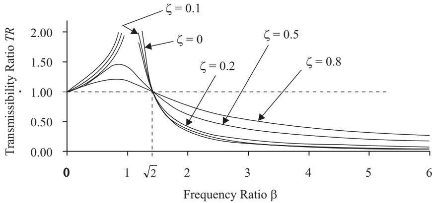
Fig. 8 Transmissibility ratio ( $TR$ ) versus frequency ratio ( $\beta$ )
