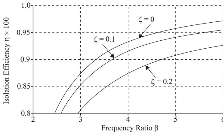
Fig. 9 Isolation efficiency  $\eta (> 80\%)$  versus frequency ratio  $\beta (> 2)$
