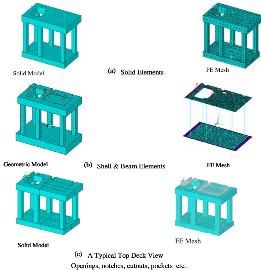
Fig. 4 Frame foundation—solid element model and shell-beam model
