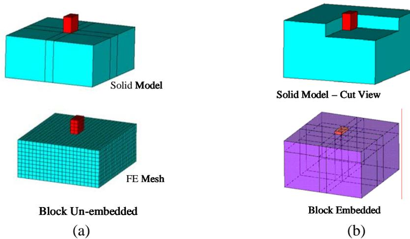
Fig. 6 Various methods of soil representation for FE modeling: (a) soil represented by a continuum below the foundation base, extending three times the width of the foundation along the length and the width and five times the depth of the foundation along the depth; (b) soil represented by a continuum starting from the ground level, extending three times the width of the foundation along the length and the width and five times the depth of the foundation along the depth
