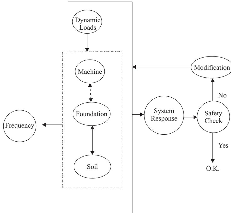
Fig. 1 Schematic diagram of a machine-foundation system subjected to dynamic loads
