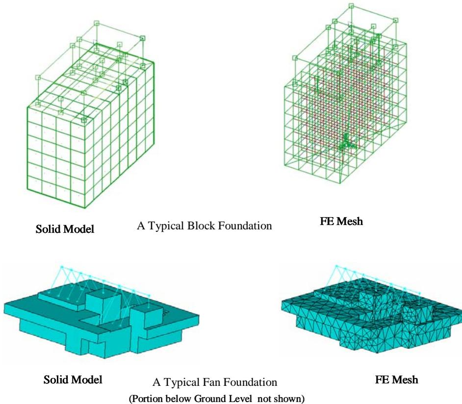
Fig. 3 Foundation block—solid model and FE mesh
