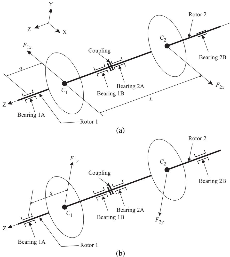
Fig. 7 Machine having two rotors with unbalanced forces out of phase in each rotor: (a) X-component of unbalanced force  $180^\circ$  out of phase; (b) Y-component of unbalanced force  $180^\circ$  out of phase
