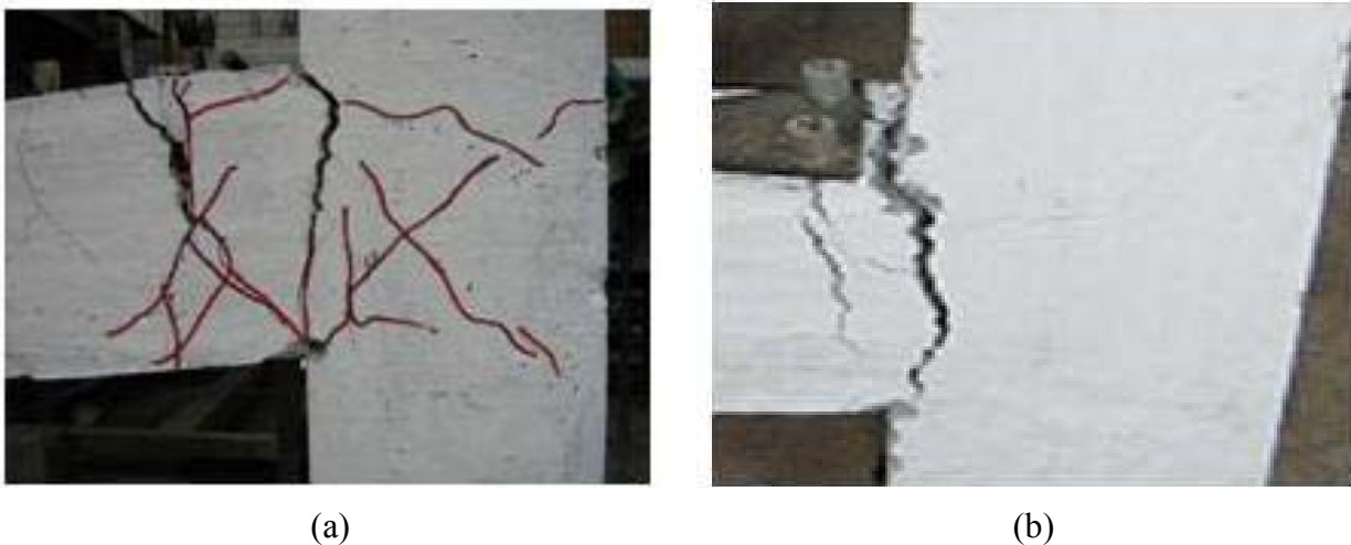
Fig. 9 Crack patterns in the specimens in the second series for (a) Specimen A2-456 and (b) Specimen A2-13920
