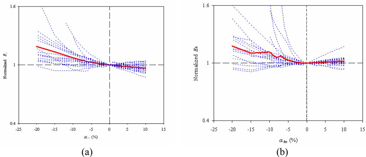
Fig. 2 Variation of hysteretic energy demand (as normalized by  $E_h$  at  $\alpha_{kn} = 0$ ) with  $\alpha_{kn}$  under 21 records (and the mean variation) for the 1st modal ESDOF systems of the (a) 20-story and (b) 9-story frames (the dashed lines represent results for the individual earthquakes and the solid line represents their mean)
