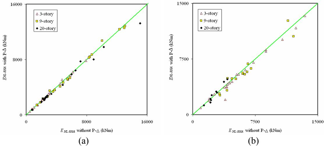
Fig. 4 Comparison of  $E_{NL-RHA}$  with and without  $P-\Delta$  effects for the (a) original SAC steel frames, and the (b) modified frames with increased stability coefficients
