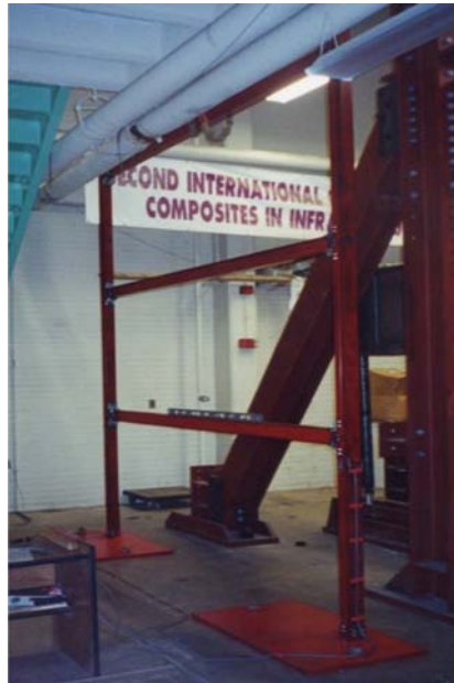
Fig. 1 Three-story experimental frame
