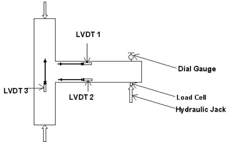
Fig. 2 Locations of LVDTs on the beam-column joint
