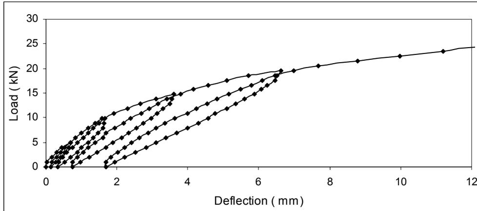
Fig. 5 Typical load-deflection plot
