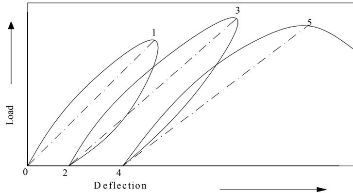
Fig. 7 The procedure adopted for determining secant stiffness
