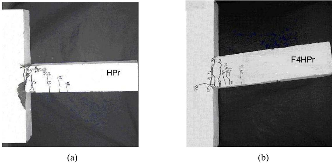
Fig. 4 (a) HPC specimen after failure; (b) SFRHPC specimen after failure
