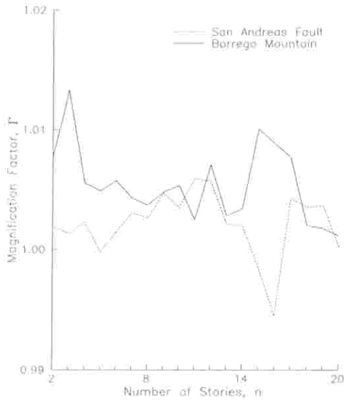
Fig.8 Effect of Concentration of Energy in Long Period Waves on Rocking Contributions at Hollywood Site.
