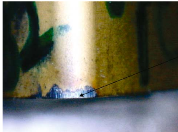
Fig. 2 Artificial flank wear created by EDM process
