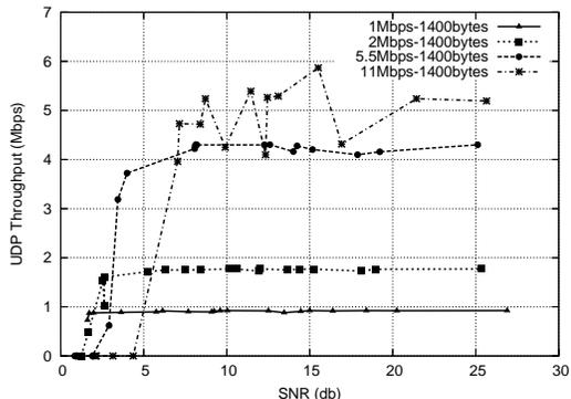
Figure 8: UDP throughput vs. SNR at 1400 bytes
