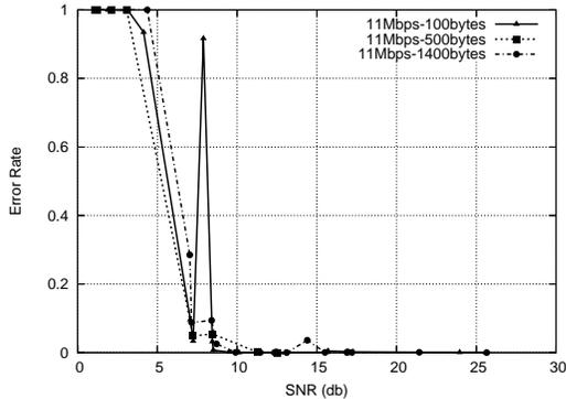
Figure 4: Error Rate vs. SNR at 11Mbps
