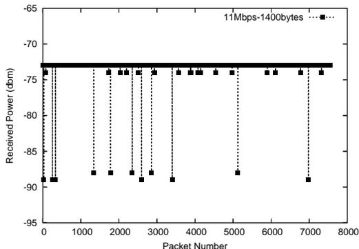
Figure 6: Signal strength variation in a long run
