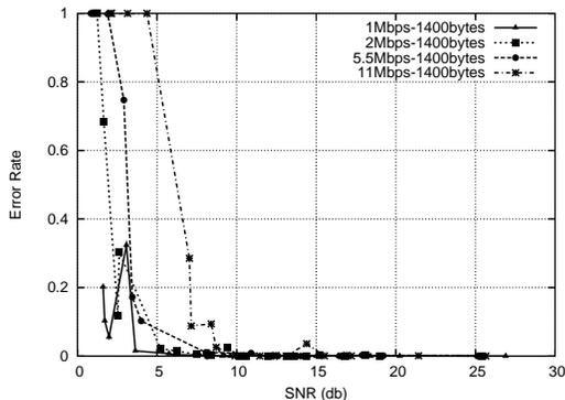
Figure 3: Error Rate vs. SNR at 1400 bytes
