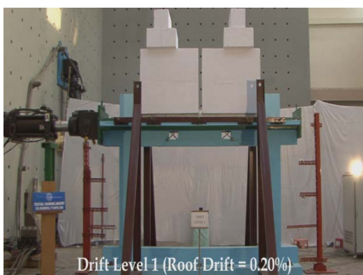
2015 Cyclic testing of 1:2.5 scaled RC frame with beam openings
