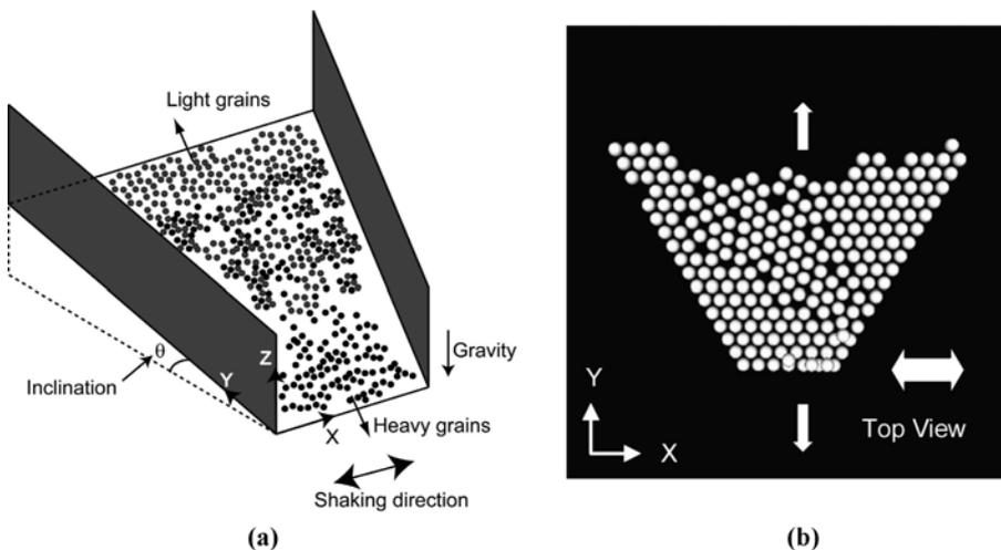
Fig. 2. (a) Three Dimensional View of Shaking Channel, (b) Initial Configuration of Grains in the Simulation
