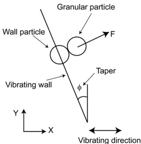
Fig. 6. Grains’ Interaction with System’s Boundary Wall
