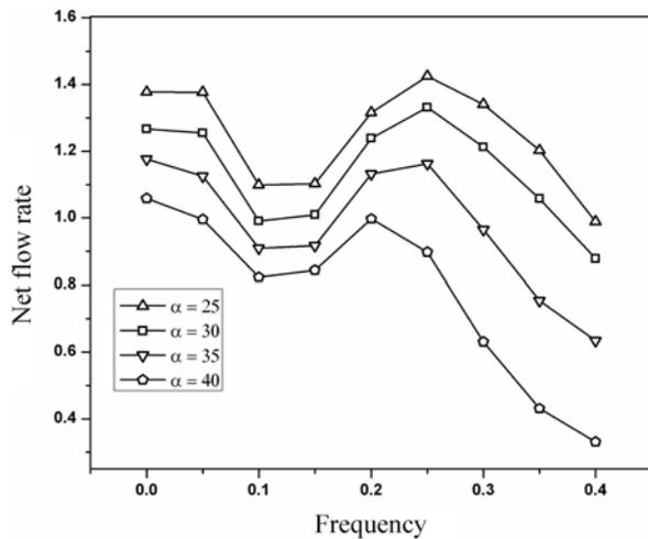
Fig. 12. Variation in the Net Flow Rate with Frequency for Different Friction Angles Keeping the Amplitude ( $A$ ) Constant at 2.0 Particle Diameters and Channel's Inclination ( $\theta$ ) at  $2^\circ$  (Friction angle ( $\alpha$ ) is in degrees and a non-dimensional frequency of 0.4 corresponds to about 10 Hz.)
