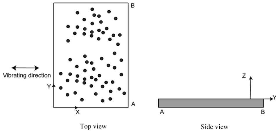
Fig. 7. Geometry of a Horizontally Vibrated Channel with Parallel Side Walls Employed in the Simulation (Channel is open at ends A and B, and not inclined to the ground.)
