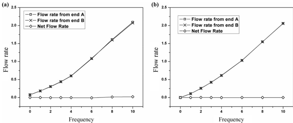
Fig. 8. Flow Rate of Particles in a Horizontally Vibrated Channel with Parallel Side Walls, Not Inclined to the Ground (The contact between grains is modeled by employing the (a) Lennard-Jones Potential, and the (b) Hertzian Contact Force Model. Vibration frequency is in Hz.)
