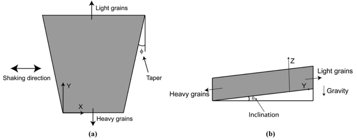
Fig. 3. Geometry of the Shaking Channel (a) Top View (b) Side View (Looking along the vibration axis)
