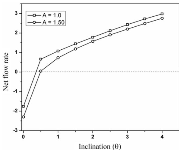
Fig. 13. Effect of Vibrating Channel's Inclination on the Net Flow Rate of Particles for Different Vibration Amplitudes at Constant Frequency of 0.4 (A non-dimensional frequency of 0.4 corresponds to about 10 hz. friction angle ( $\alpha$ ) is kept at  $26.56^\circ$  ( $\mu=0.5$ ) and inclination angle is in degrees.)
