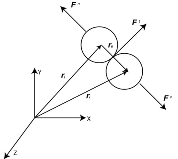
Fig. 4. Contact between Two Particles
