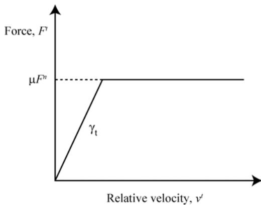
Fig. 5. Coulomb Friction Model: A Limiting Friction Force to Prevent Sliding between Particles
