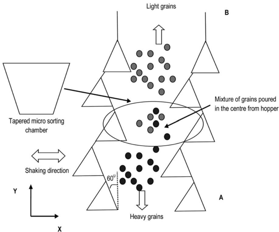
Fig. 1. The Geometry of a Segregating Channel in an Actual Grain Sorter (End A is at lower elevation than end B.)
