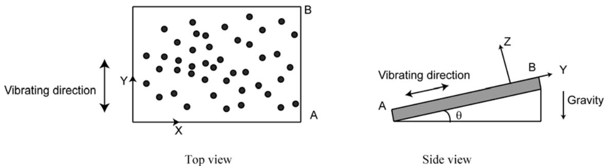
Fig. 9. Experimental Setup of Blair and Kudrolli (2003), cf. Fig. 1 ( Top (B) and bottom (A) ends of vibrating plate are closed, i.e., there is no influx or efflux of grains in the system.)
