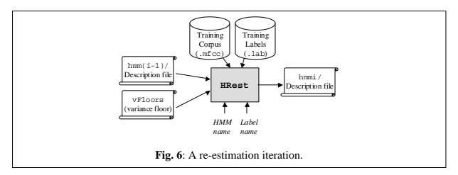
The following command line perform one re-estimation iteration with HTK tool HRest, estimating the optimal values for the HMM parameters (transition probabilities, plus mean and variance vectors of each observation function):
