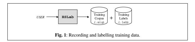
First, we have to record the "Yes" and "No" speech signals with which word models will be trained (the *training corpus*). Each speech signal has to be labelled, that is: associated with a text (a label) describing its content. Recording and labelling can be done with the HSLab HTK tool (but any other tool could be used).
