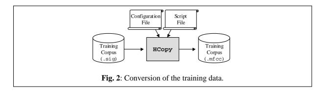
The speech recognition tools cannot process directly on speech waveforms. These have to be represented in a more compact and efficient way. This step is called "acoustical analysis":
