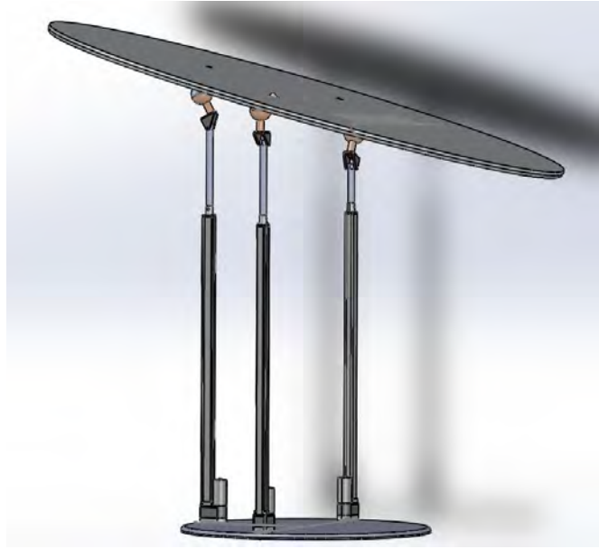
Fig. 5 Platform's final Configuration
