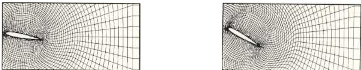
Figure 7. Flow past an oscillating NACA 0012 airfoil at Reynolds number 1,000: mesh at 10° and 30° angle of attack
