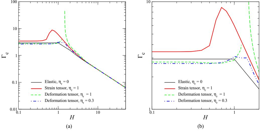
FIG. 3. Plane Couette flow past a deformable solid. (a) Critical strain rate as a function of thickness  $H$  for different  $\eta_r$ . (b) Zoomed in view of (a) for smaller values of  $H$ .
