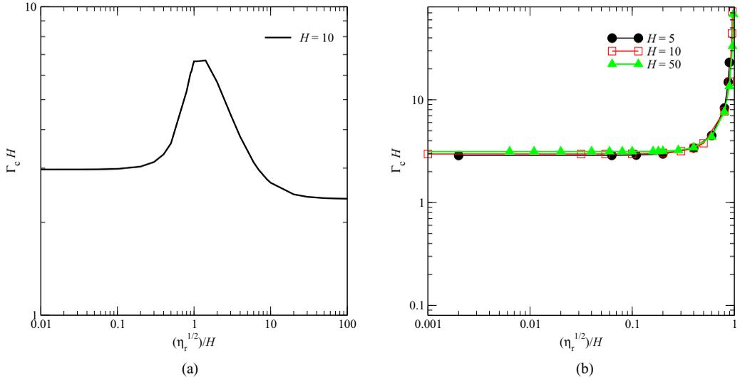
FIG. 4. Plane Couette flow past a deformable solid. Scaling of  $\Gamma_c$  with  $\eta_r$  for  $H \gg 1$  is shown for the two different formulations of viscous effects in the solid: (a) strain-rate-tensor formulation and (b) rate-of-deformation tensor formulation.
