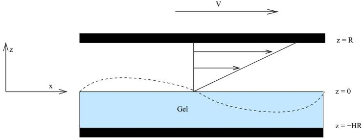
FIG. 1. Schematic representation of plane Couette flow past a deformable solid and the (dimensional) coordinate system used.
