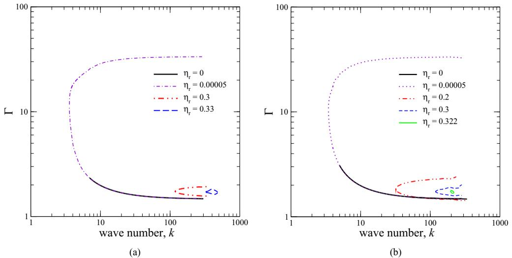
FIG. 5. Pressure-driven flow in a channel with deformable walls in the creeping-flow limit and the effect of the solid-fluid viscosity ratio  $\eta_r$  on the neutral stability curves for (a)  $H = 0.5$  and (b)  $H = 1$ . The short-wave instability is stabilized with an increase in  $\eta_r$  and the instability eventually disappears after a critical  $\eta_r$ .
