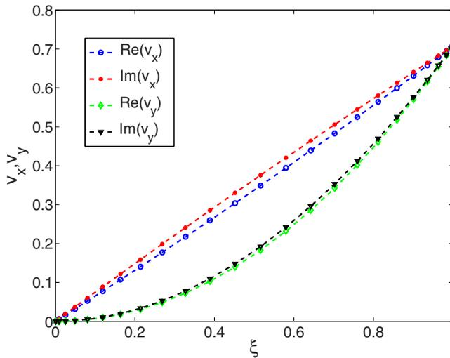
FIG. 9. Eigenfunction plots for the streamwise and normal components of the velocity for the neutrally stable eigenvalue  $c = 0.950578$  obtained at  $\text{Re} = 0$ ,  $H = 15$ ,  $y_0 = 0.01$ ,  $k = 0.0835$ , and  $\Gamma = 0.17141$ .
