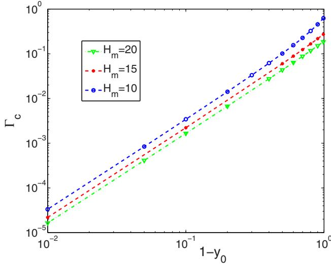
FIG. 8. Variation of  $\Gamma_c$  with  $y_0$  for constant  $\tilde{H} = (1 - y_0)H$  at  $\text{Re} = 0$ . The figure shows scaling  $\Gamma_c \sim (1 - y_0)$ .
