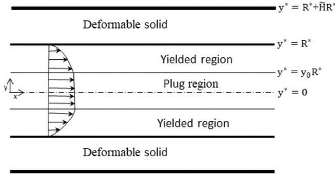
FIG. 1. Schematic of the flow geometry studied in the present work. Here  $y_0 R^*$  and  $\bar{H}R^*$  are, respectively, the dimensional plug and solid thicknesses. At  $y^* = R^* + \bar{H}R^*$  and  $-R^* - \bar{H}R^*$ , the deformable solid is perfectly bonded to a rigid solid.
