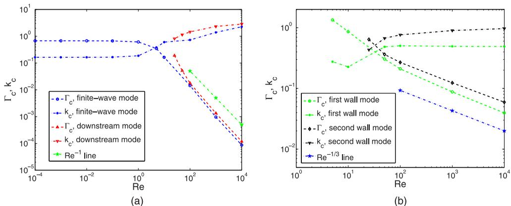
FIG. 13. Variation of critical parameters with  $Re$  at  $H = 5$  and  $y_0 = 0.01$  for (a) inviscid and (b) wall modes. The finite-wave mode is the most unstable inviscid mode while the first wall mode is the most unstable wall mode.
