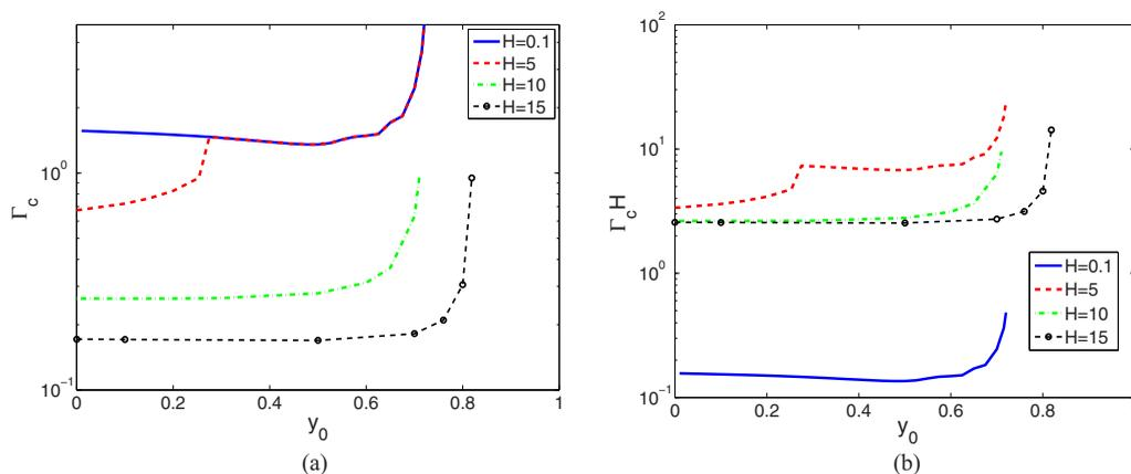
FIG. 7. (a) Variation of  $\Gamma_c$  with  $y_0$ . (b) Collapse of the data for  $H = 10$  and  $15$  shows the existence of the scaling  $\Gamma_c \sim 1/H$  for the finite-wave instability ( $\Gamma_c H$  vs  $y_0$ ).
