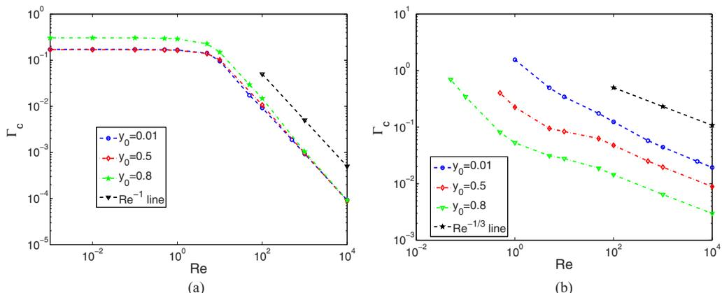
FIG. 17. Variation of  $\Gamma_c$  with  $Re$  at  $H = 15$  for (a) finite-wave and (b) first wall modes. The finite-wave mode is the most unstable inviscid mode while first wall mode is the most unstable wall mode.
