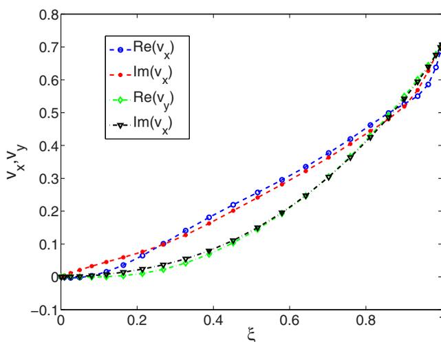
FIG. 14. Eigenfunction plots for the streamwise and normal components of the velocity for the neutrally stable eigenvalue  $c \sim 0.953744 + 0i$  obtained at  $Re = 1000$ ,  $H = 5$ ,  $y_0 = 0.01$ ,  $k = 1.392$ , and  $\Gamma = 0.0009635$ .
