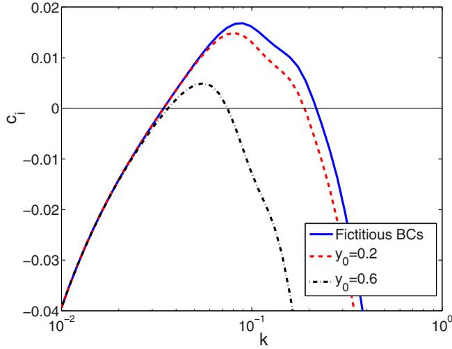
FIG. 5. Variation of  $c_i$  with  $k$  of the most unstable mode at  $\text{Re} = 0$ ,  $\Gamma = 0.5$ , and  $H = 10$ . In the limit of  $y_0 \rightarrow 0$ , the finite-wave instability predicted here approaches the results for stability of plane Poiseuille flow of a Newtonian fluid with fictitious no-slip boundary conditions  $\tilde{v}_x = 0$  and  $\tilde{v}_y = 0$  at the channel centerline.
