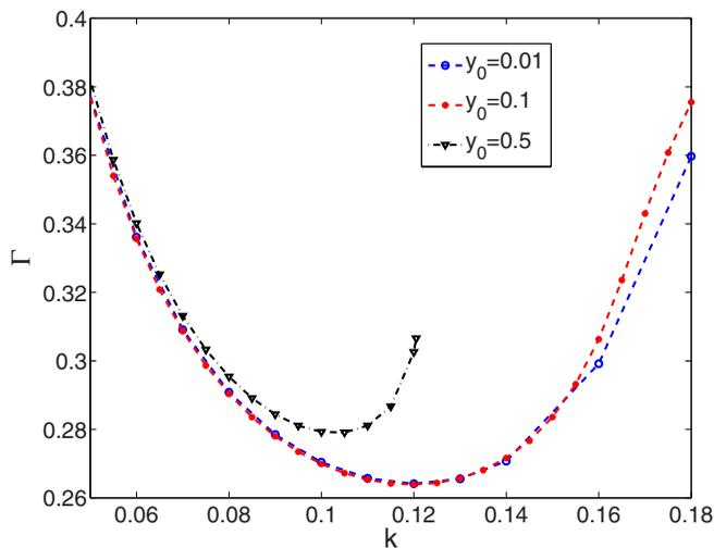
FIG. 3. Neutral stability curve in  $k$ - $\Gamma$  space for  $\text{Re} = 0$  and  $H = 10$ . The figure shows the existence of the finite-wave instability for the Bingham fluid absent for the Newtonian fluid.
