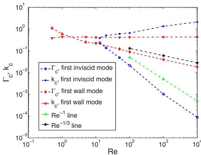
FIG. 16. Variation of critical parameters ( $\Gamma_c$  and  $k_c$ ) with  $Re$  at  $H = 5$  and  $y_0 = 0.5$  for inviscid and wall modes. The inviscid and wall modes are, respectively, the critical modes of instability for  $Re < 10$  and  $Re > 10$ .
