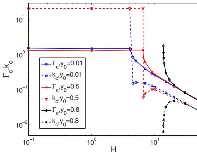
FIG. 6. Variation of  $\Gamma_c$  and  $k_c$  with  $H$  for  $\text{Re} = 0$ . The finite-wave and short-wave instabilities are the critical modes of instability in  $H > 1$  and  $H < 1$  regions, respectively.
