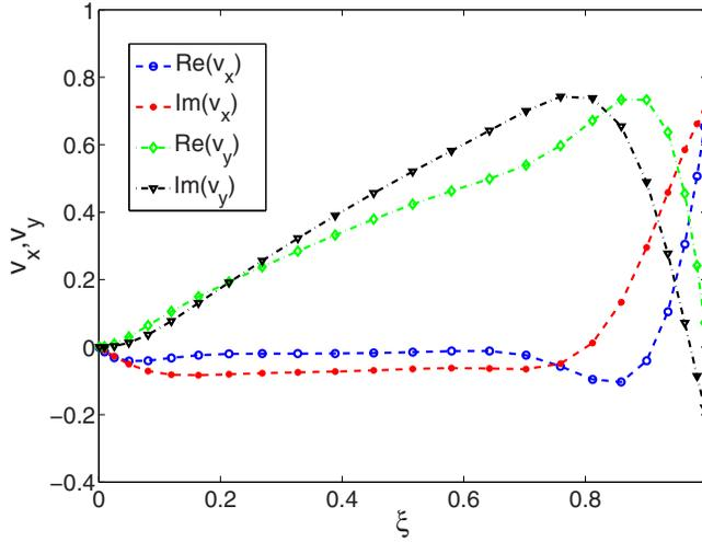
FIG. 15. Eigenfunction plots for the streamwise and normal components of the velocity for the eigenvalue  $c \sim -0.201800 + 0i$  obtained at  $Re = 1000$ ,  $H = 5$ ,  $y_0 = 0.01$ ,  $k = 0.494$ , and  $\Gamma = 0.08767$ . The maximum variation of the eigenfunctions near the deformable wall indicates the wall mode nature of the upstream mode.
