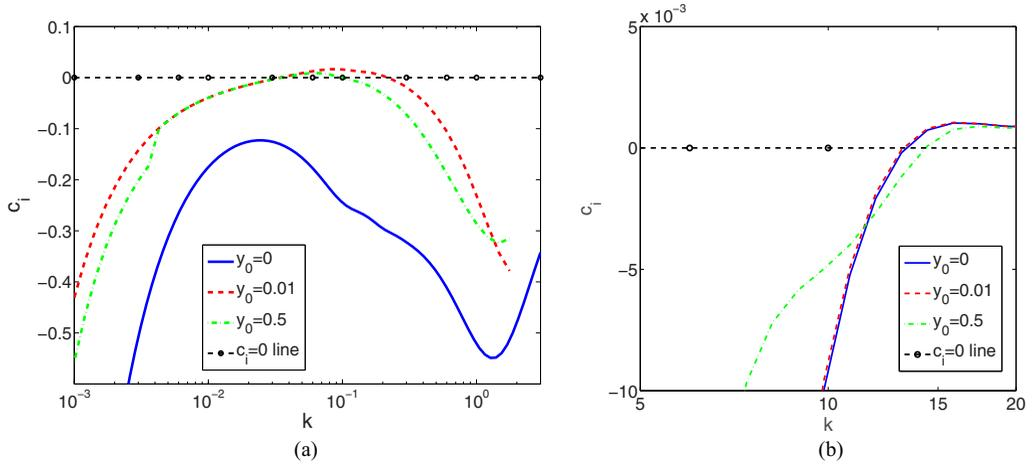
FIG. 2. Variation of  $c_i$  of the most unstable eigenvalue with  $k$  for  $T = 0$  and  $\text{Re} = 0$ . Here  $y_0 = 0$  defines a Newtonian fluid (varicose mode). The presence of (a) finite-wave instability for  $H = 10$  and  $\Gamma = 0.5$  ( $k < 1$ ) and (b) short-wave instability for  $H = 0.1$  and  $\Gamma = 2$  ( $k > 5$ ) is shown for pressure-driven flow of a Bingham fluid in the creeping-flow limit.
