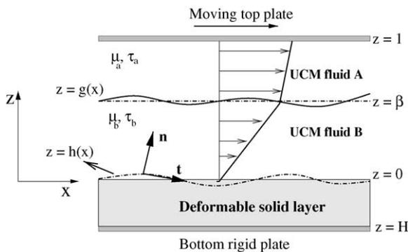
Fig. 1. Schematic diagram showing the configuration and (non-dimensional) coordinate system considered in Section 2: Two UCM fluids with viscosities  $\mu_a$  and  $\mu_b$ , and with relaxation times  $\tau_a$  and  $\tau_b$  flowing past a deformable solid layer.
