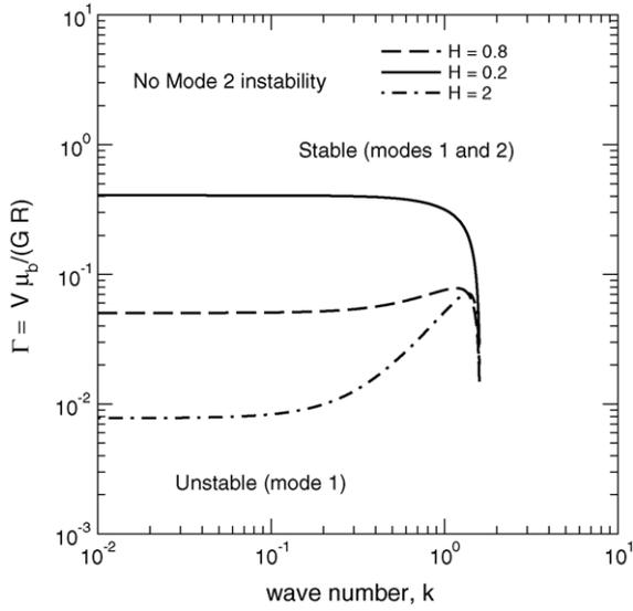
Fig. 7. Effect of solid layer thickness  $H$  on the stabilization of two-fluid interfacial instability by the deformable solid layer: neutral stability curves in the  $\Gamma$ - $k$  plane. Data for  $W_a = 1$ ,  $W_b = 2$ ,  $Re = 1$ ,  $\mu_r = 0.25$ ,  $\beta = 0.4$ ,  $\eta_r = 1$ ,  $\Sigma = 0.1$ .
