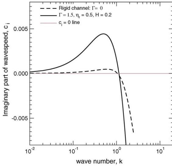
Fig. 3. Destabilization of the two-fluid interfacial mode by the deformable solid layer:  $c_i$  vs.  $k$  for  $W_a = 0.5$ ,  $W_b = 1$ ,  $\beta = 0.4$ ,  $Re = 1$ ,  $\Sigma = 0.1$ , and  $\mu_r = 1.5$ .
