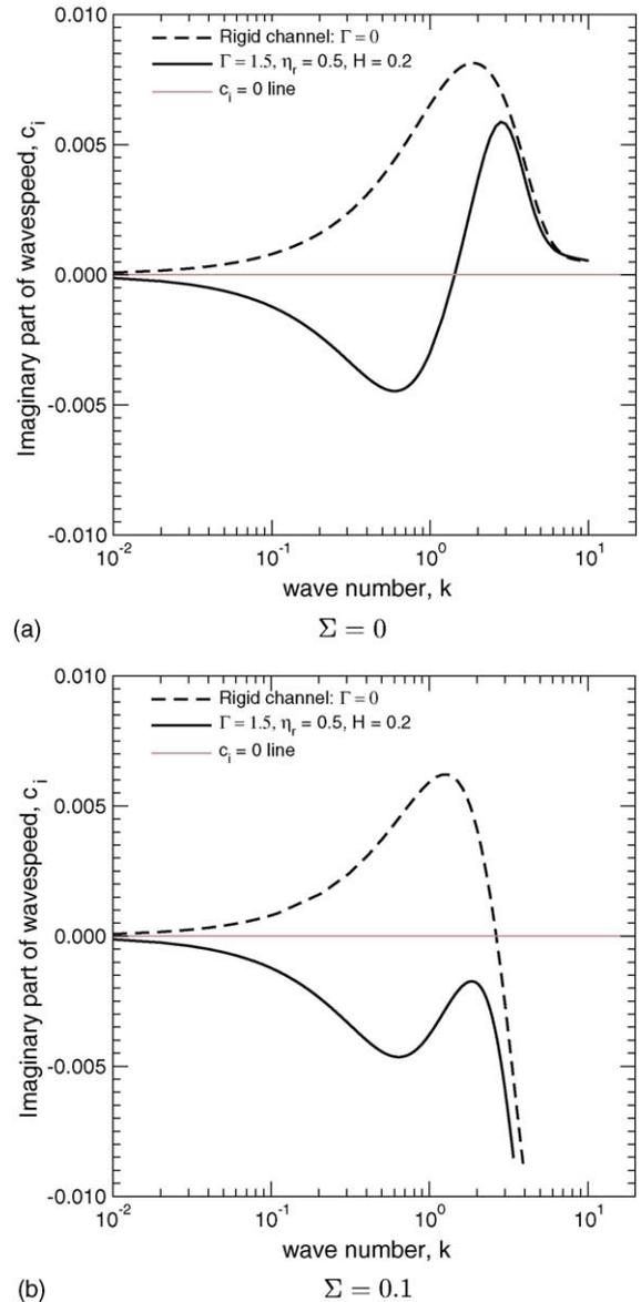
Fig. 2. Stabilization of the two-fluid interfacial mode by the deformable solid layer, while it is unstable in a rigid channel:  $c_i$  vs.  $k$  for  $W_a = 0.5$ ,  $W_b = 1$ ,  $\beta = 0.4$ ,  $\mu_r = 0.5$ ,  $Re = 1$  for  $\Sigma = 0$ , and  $\Sigma \neq 0$ .
