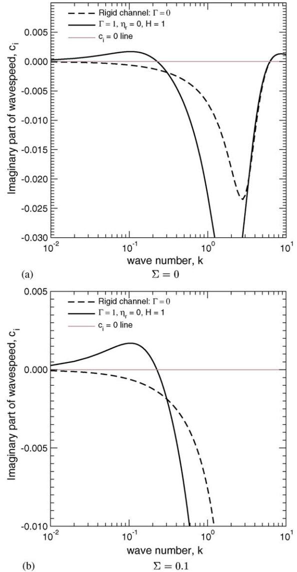
Fig. 4. Destabilization of the two-fluid interfacial mode by the deformable solid layer while it is stable in a rigid channel:  $c_i$  vs.  $k$  for  $W_a = 0.5$ ,  $W_b = 1$ ,  $\beta = 0.7$ ,  $Re = 1$ , and  $\mu_r = 0.5$  for  $\Sigma = 0$  and  $\Sigma \neq 0$ .
